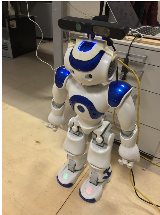
Figure 5.1. The figure shows NAO v5 humanoid robot, the platform used for the experiments of this thesis, equipped with an ASUS Xtion Pro RGB-D camera. The camera is connected via USB to an external computer which runs elevation_mapping and the footstep planner. The external computer communicates with NAO through an ethernet cable using TCP.
